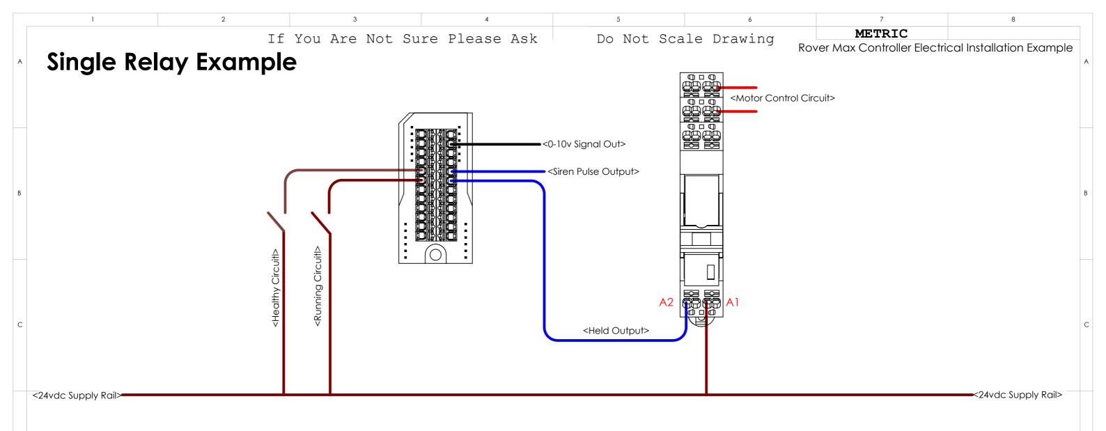
A1 - High Side of Coil A2 - Low Side Of Coil
